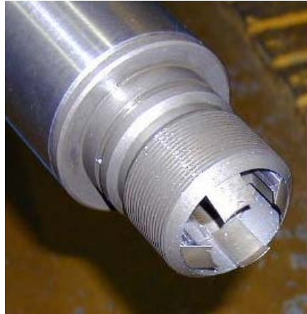
Figure 3 – Cable Shearing Mechanism
